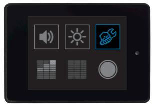
The interference level on the antenna is displayed in 10 steps.
