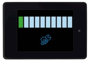
The signal blocks on the display indicate the amount of interference being received by the antenna. An acoustic signal corresponds to the number of signal blocks on the display. This facilitates finding a location free of interference for the antenna when the display is not visible.
